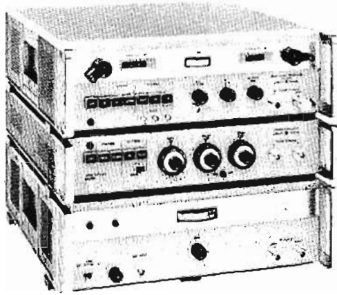
Figure 1. Full rack width cabinets stack one atop the other.
