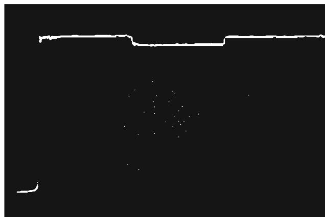
Figure 2. TDR display of a section of unknown cable spliced into a length of 50-ohm cable. Noting the distance setting of 40 cm/cm, and reflection coefficient sensitivity of 0.2/cm, one can determine the unknown cable is 120 cm long and has a Z_0 of 44 ohms. Impedance changes as small as 0.1 ohm are readily resolved when magnified.
