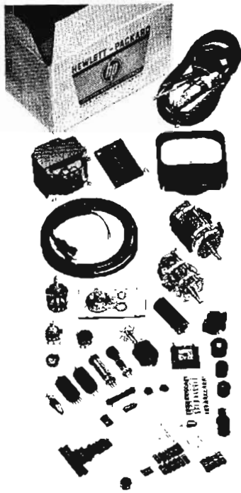
These items make up an "Isolated Service Kit" for the Model 410B Vacuum Tube Voltmeter.
